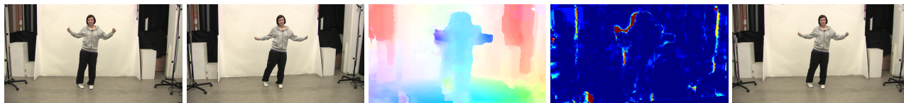
Figure 1: Belief Propagation Optical Flow. Left to right: two 1920 \times 1080 input images A and B , optical flow from A to B , flow symmetry and rendered result. We specifically tailored our optical flow for image morphing in the presence of large motion and occlusions. We incorporate recent advances in computer vision to produce visually convincing results.
